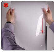
Slide the white backing sheet into the channels in the light box frame.
