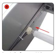
Locate the fluorescent tube terminals into the connector cups attached to the frame.
