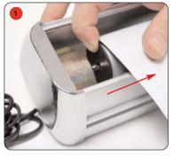
Remove the drive roller (B) from the drive unit, pushing it towards the spring end of the drive unit.
