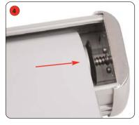
Locate the drive roller into the spring end of the drive unit, compress the spring and fit other end of drive roller.
